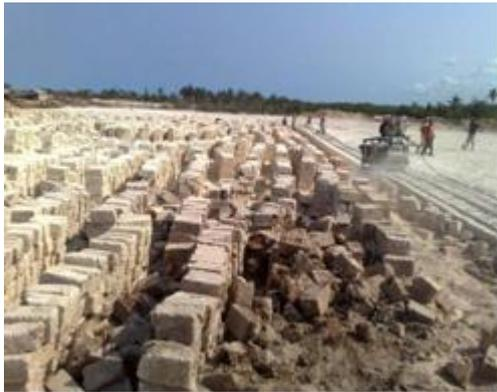
**Figure 6** – Stone cutting for building from limestone bed rock in Kilifi, Coast Province, Kenya.
